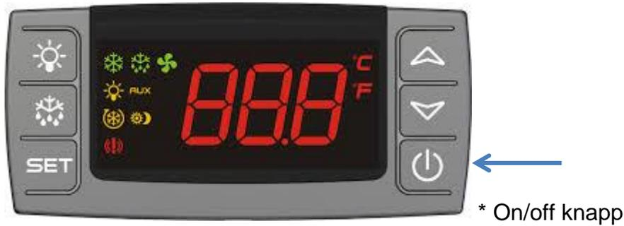
1. Connect the power cable to an earthed electrical socket (230-240 V~) and press \*on at the on/off-button to start the heating process.
